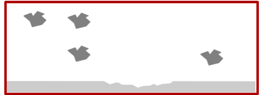
Erosive wear caused by impact of particles
