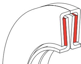
We are using labyrinth seal, which is a mechanical seal that fits around the axle or shaft to prevent the leakage of any particles.
