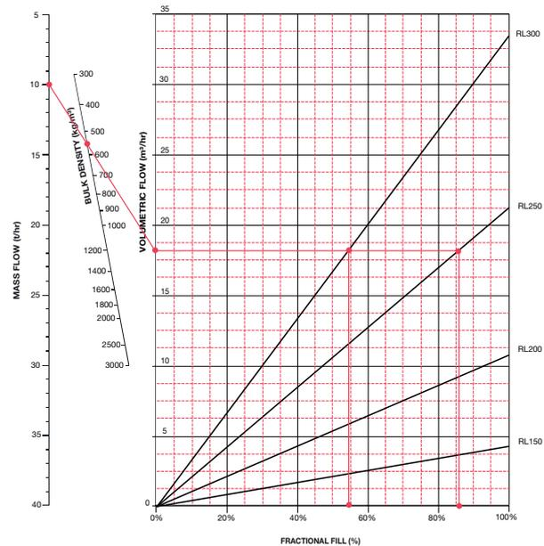
EXAMPLE: A MATERIAL WITH A BULK DENSITY OF 550KG/M<sup>3</sup> AND REQUIRED CAPACITY OF 10T/HR CAN BE ACHIEVED BY RL 250 & AT 86% FILLING CAPACITY WITH 31 RPM AND ALSO BY RL 300 AT 54% FILLING CAPACITY WITH 28 RPM.
